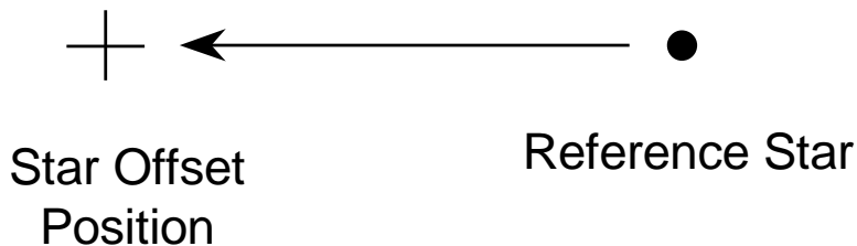
Figure 1. By calculating the appropriate star offset position, we can make a precise alignment correction by recentering the star via the mount’s altitude or azimuth adjustment mechanism.
